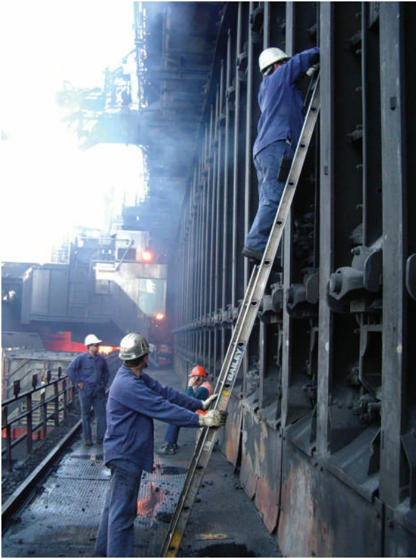
Figure 1. Specialists adjusting battery doors (Down et al., 2006, p. 102; reprinted with permission).
